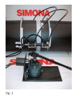
A 40 V standard automatic welding machine for electrofusion sockets can then be connected.
